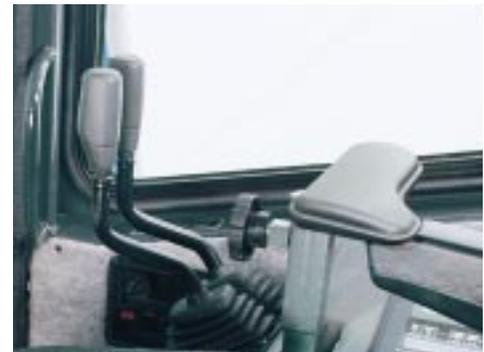
**Kick-down switch is conveniently located** on the boom lever. A simple motion of the thumb actuates this valuable productivity feature.
